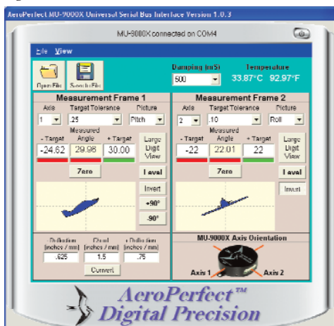
Sometimes, you get lucky! The green lights tell me that I am within my set target tolerance. The numbers show me I am well within them! Note the calculator on the bottom of the left side of the screen. I've set it for 5/8-inch down deflection and 3/4-inch up with a 1.5-inch control-surface chord. The calculator determined the actual angles and automatically entered them as the targets in frame 1.
