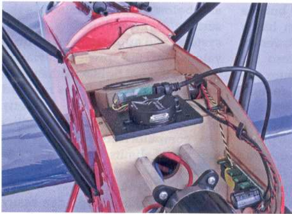
◀ The holes on the measuring head unit holder allow secure attachment to propeller adapters for motor thrust angles.
