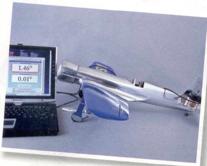
After establishing a neutral reference point, the measuring head is placed upon the flat plate stabilizer of this 32-in. wingspan Hughes racer and the incidence shown on the screen is 1.46 degrees
