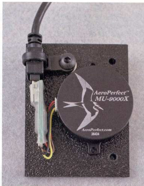
Closeup of the two axis measuring head unit.
