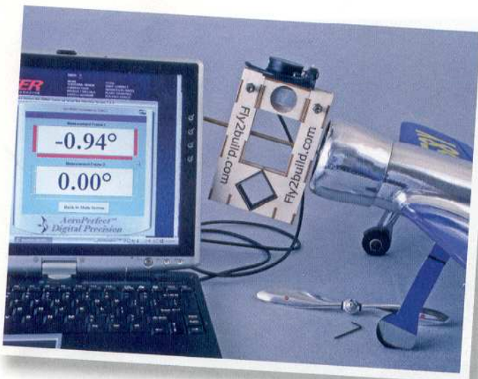
➤ The motor down thrust is measured by using a piece of snug fitting brass tubing slipped over the motor shaft and attached through the jigs and is indicated as .94 degrees.
