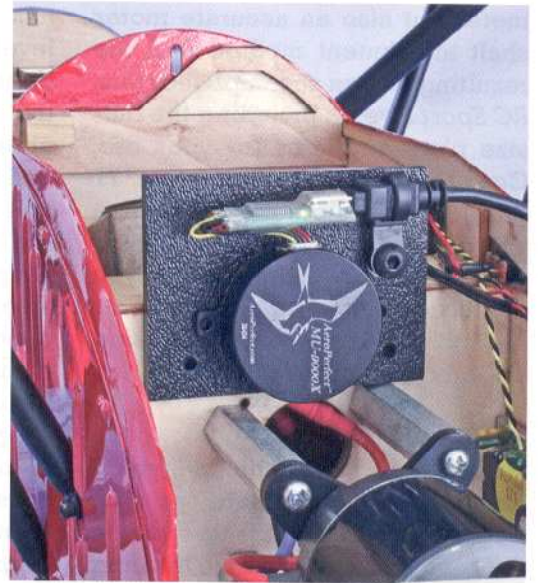
▶ After subtracting 90 degrees from the previously measured neutral angle, the measuring head is rotated 90 degrees positive to determine the firewall thrust angle.
