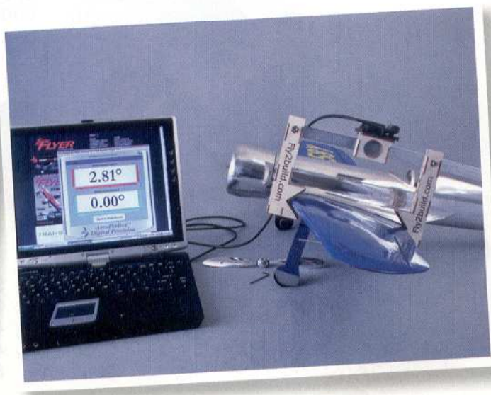
The wing incidence is measured next and the resulting angle is 2.81 degrees of positive incidence relative to the neutral reference point. The gig is offered as a plan on the rc-sf.com Web site.
